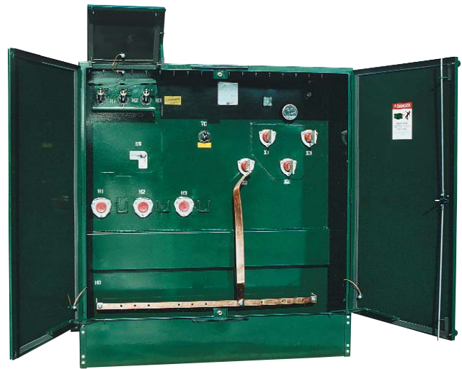
1500KVA Dead Front Radial Feed 3 phase Pad-Mounted 24.9kVGY/14.4 kV - 600Y/347V
